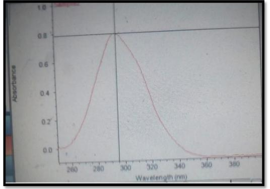
Fig 2: UV Visible spectra Pure Embelin
