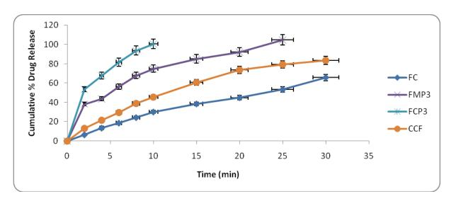
Fig 1:Comparative Cumulative % Drug Release Versus Time Plots (Zero-order) of Promising Fast Dissolving Tablet Formulations, Control and Conventional Commercial Formulations (CCF) in pH 6.8 Phosphate
