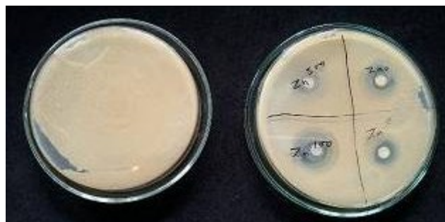
Fig. 4: Disc Diffusion Method for antibacterial activity at different calcinated temperature for ZnO
