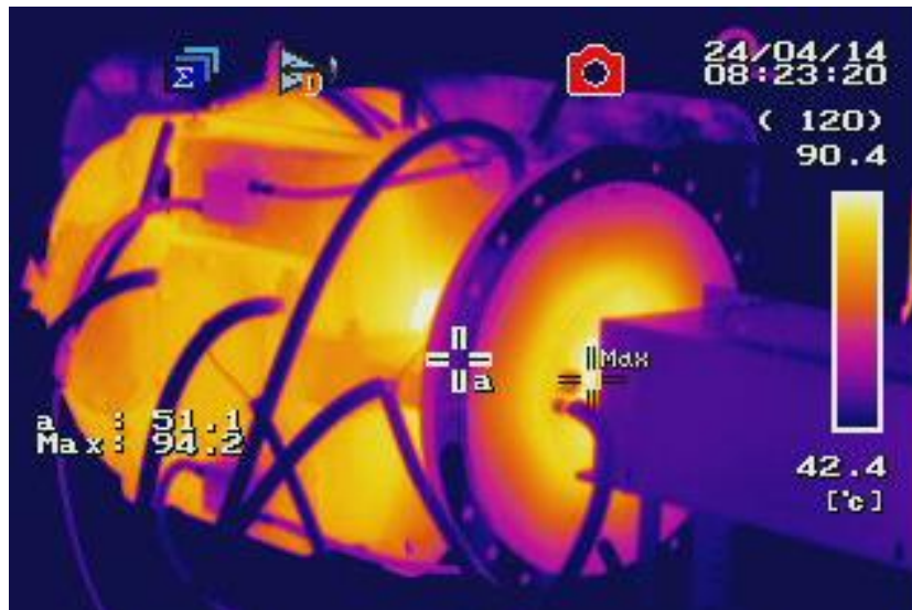
Fig. 2. Examples of thermograms obtained for the mining right-angle spur planetary gearbox
