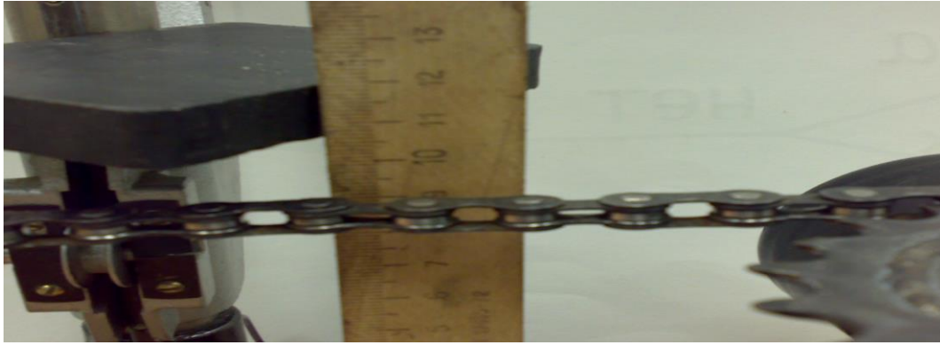
Fig. 5. Other foreshortening when we can see as the magnet raised slightly the line of the chain and put it in one plane with sprocket
