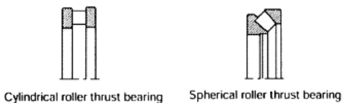
Fig.8 – Types of roller bearings used in the construction of gas turbines [13,pg. 470]
