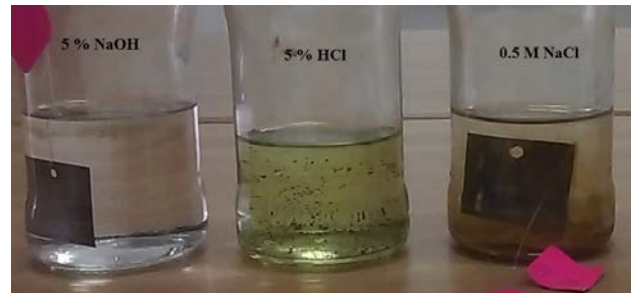
Figure 12. Visual aspect of steel S220GD after 28 days of immersion in corrosive environments
