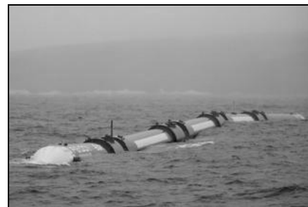
Fig. 9 Pelamis Wave Energy Converter Orkney, U.K
