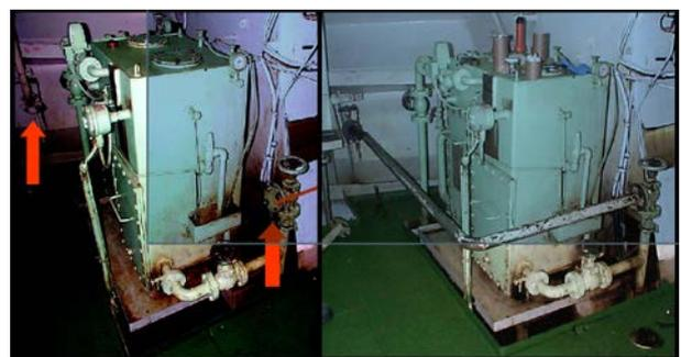
**Fig.4 Direct discharge; bypassing the oily-water separator system**
