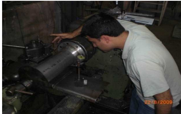
Figure 3. The measuring of angular distortion.
