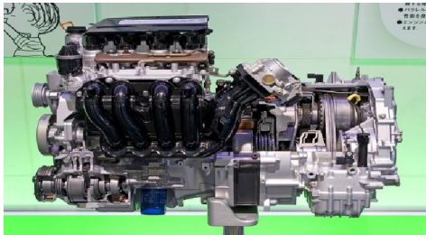
Fig.-14(a): Image of i-VTEC engine
