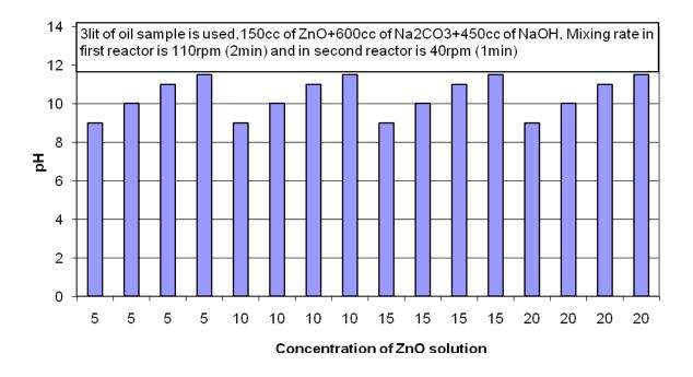
Figure 2. pH versus ZnO concentration
