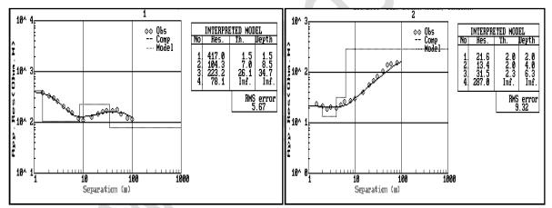
Figure 2 Geo resistivity curve of location 1
