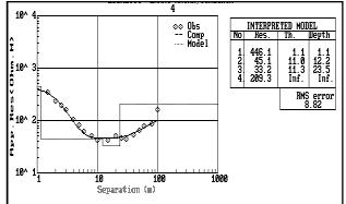
Figure 5 Geo resistivity curve of location 4
