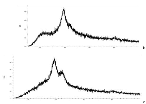
Fig(3) X-ray diffraction spectra of a: PVA b:chitosan c:PVA/CCblend
