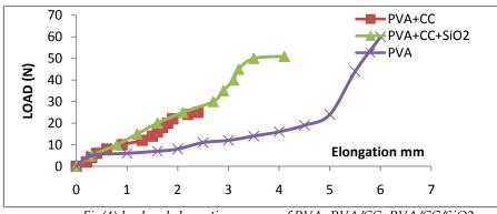
Fig(4) load and elongation curves of PVA, PVA/CC, PVA/CC/SiO2
