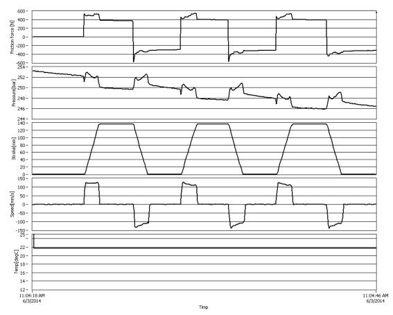
Fig. 13. The complex characteristic graphs for pressure step values of 250 bar.
