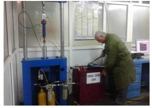
(b) Creating pressure with the hand Pump Fig. 3. The stand for experimental determination of frictional forces.
