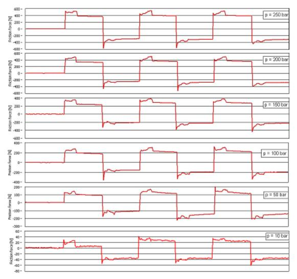
Fig. 15. The variations of the friction forces for all pressure steps
