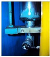
Fig. 7. The stroke transducer
