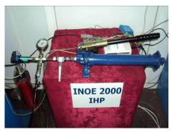
Fig. 9. The hand oil pump
