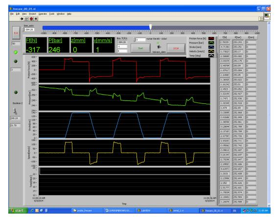
Fig. 14. The screen of the computer for 250 bar.
