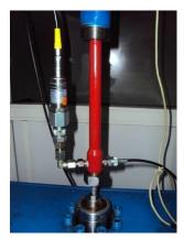
Fig. 5. The pressure and temperature transducer.
