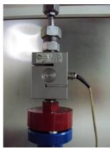
Fig. 6. The force transducer.
