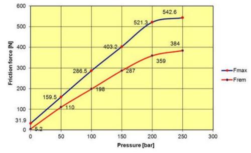
Fig. 16. The variation of the friction forces versus the pressure.
