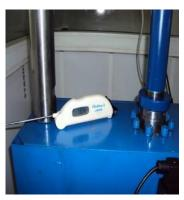
Fig. 8. The ambiental thermometer
