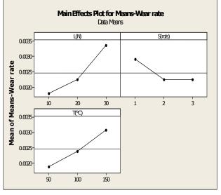
Fig. 2. Main effects plot for Means-Wear rate.
