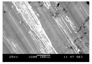
Fig. 6. SEM Micrograph for L=20 N, S=1 m/s, T=100 °C.
