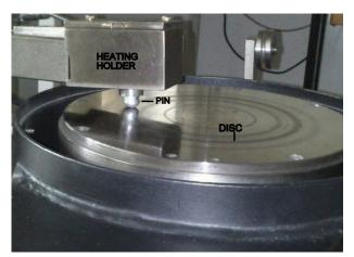
Fig. 1. Pin-on-disc wear tester.
