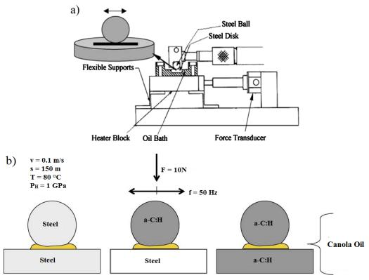
Fig. 1. HFRR test: a) schematic diagram of HFRR, b) materials and experimental condition.
