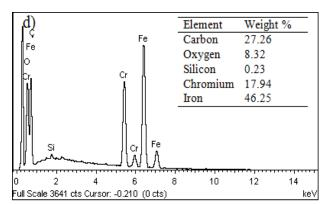
**Fig. 5.** EDS analysis of the balls surfaces a) as deposited a-C:H DLC films; and worn surfaces when lubricated with Canola oil: (b) steel/steel (c) steel/a-C:H and (d) a-C:H/a-C:H combination.
