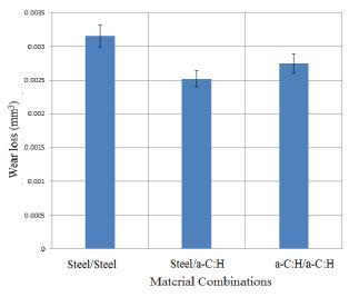
**Fig. 3.** Wear loss of selected ball and disc sets of steel/steel, steel/a-C:H and a-C:H/a-C:H material combinations, when lubricated with Canola oil. Error bars represent  $\pm$  one standard deviation of the measurements.
