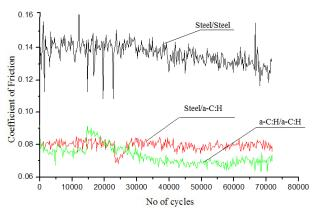
**Fig. 2.** Coefficient of friction of steel/steel, steel/a-C:H and a-C:H/a-C:H combinations with Canola oil lubrication.
