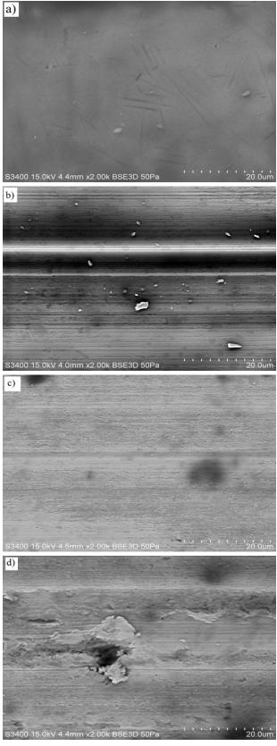
**Fig. 4.** SEM micrographs of the balls surfaces a) deposited surface of a-C:H DLC films; and worn surfaces when lubricated with Canola oil: (b) steel/steel (WSD =  $416\pm 1.6 \mu$ m) (c) steel/a-C:H (WSD =  $318\pm 1.3 \mu$ m) and (d) a-C:H/a-C:H combination (WSD =  $355\pm 1.1 \mu$ m).
