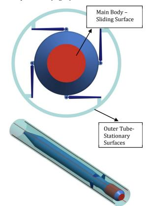
**Fig. 1.** Cross-sectional view and complete assembly under consideration.
