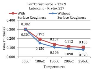
**Fig. 9.** Effect of surface roughness at 32KN Force for Krytox 227.
