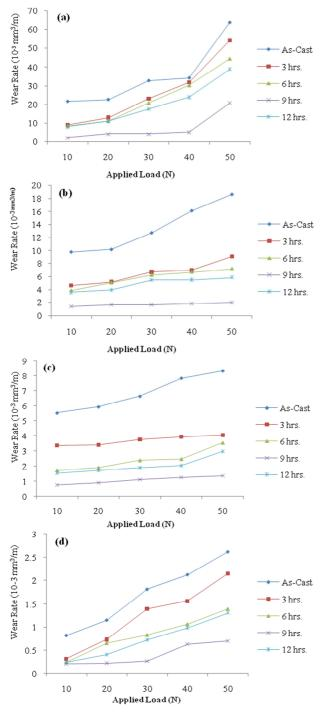
**Fig. 3.** Cumulative wear rate of as-cast and different ageing treated composites as a function of load when sliding speed of 3.77 m/s and sliding distance of 4500 m. (a). A356 alloy (b). A356-3%SiC<sub>p</sub>-3%Gr (c). A356-6%SiC<sub>p</sub>-3%Gr (d). A356-9%SiC<sub>p</sub>-3%Gr.
