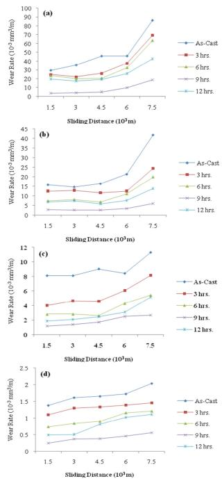
**Fig. 1.** Cumulative wear rate of as-cast and different ageing treated composites as a function of sliding distance at constant sliding speed of 3.77 m/s and applied load of 30 N. (a). A356 alloy (b). A356-3%SiC<sub>p</sub>-3%Gr (c). A356-6%SiC<sub>p</sub>-3%Gr (d). A356-9%SiC<sub>p</sub>-3%Gr.
