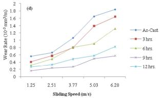
**Fig. 2.** Cumulative wear rate of as-cast and different ageing treated composites as a function of sliding speed at constant sliding distance of 4500 m and applied load of 30 N. (a). A356 alloy (b). A356-3%SiC<sub>p</sub>-3%Gr (c). A356-6%SiC<sub>p</sub>-3%Gr (d). A356-9%SiC<sub>p</sub>-3%Gr.
