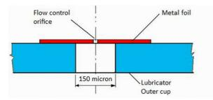
Fig. 7. Arrangement of flow control orifice.
