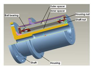
Fig. 2. Bearing cartridge assembly.
