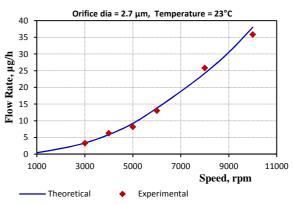
**Fig.10.** Variation of theoretical and experimental flow rate with operating speed.
