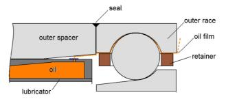
Fig. 6. Schematic view of oil flow from the lubricator.
