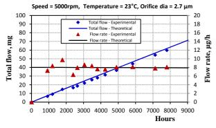
Fig. 9. Theoretical and experimental results of a lubricator with 2.7  $\mu m$  diameter orifice.
