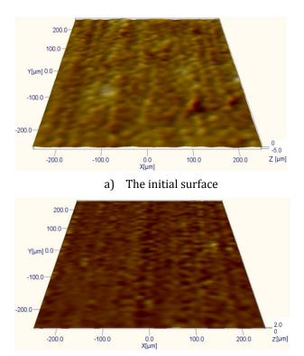
b) The worn surface (F = 5 N, v = 0.25 m/s, L = 7500 m) **Fig. 2.** Virtual images of the polymeric blocks made of PBT + 10 % PTFE.
