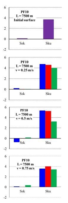
**Fig. 4.** The influence of the normal force on the average values of the dimensional amplitude parameters for the blocks made of PF10.
