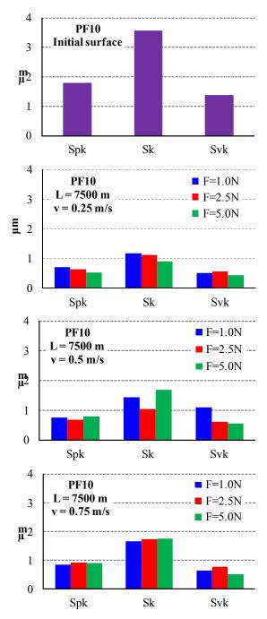
**Fig. 4.** The influence of the normal force on the average values of the 3D functional parameters for the blocks made of PF10.
