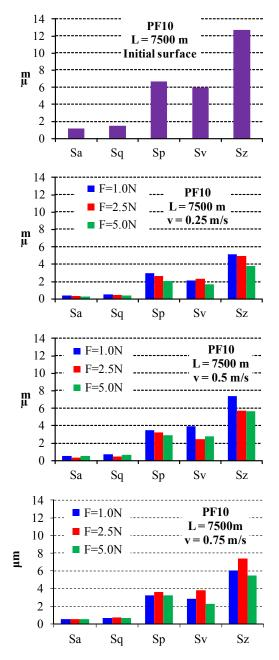
**Fig. 3.** The influence of the normal force on the average values of the dimensional amplitude parameters for the blocks made of PF10 (PBT + 10 % PTFE).
