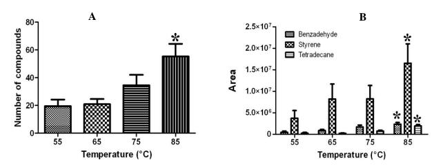
Figure 2. Effect of temperature on the number of compounds released from EPS-based products (A), and on the peak area for specific compounds (B). \*Significantly different as compared to 55 °C (P < 0.05).
