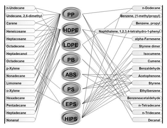
**Figure 3.** Compounds identified in different plastic-based products (3,4,8,19,14,15,20). PP: Polypropylene, HDPE: High density polyethylene, LDPE: Low density polyethylene, PB: Polybutylene, ABS: Acrylonitrile-Butadiene-Styrene, PS: Polystyrene, EPS: Expanded polystyrene, HIPS: High-impact polystyrene.
