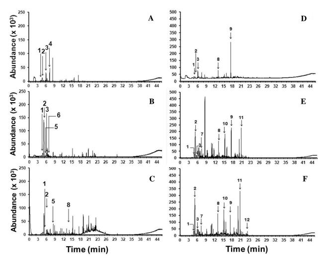
**Figure 1.** Typical SPME-GC/MS chromatograms of EPS-based products. Soup containers (**A**, **D**), food containers (**B**, **E**) and plates (**C**, **F**) at extraction temperatures of 55 °C and 85 °C, respectively. 1. Ethylbenzene. 2. Styrene. 3. Benzaldehyde. 4. Benzene, (1,1-dimethylethoxy). 5. Cumene. 6. Benzene, (1-methylpropyl). 7. Acetophenone. 8. Tetradecane. 9. Diethyl Phthalate. 10. Pentadecane. 11. Benzene, 1,1'-(1,2-cyclobutanediyl)bis, trans. 12. Nonanal.
