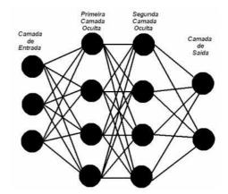
Figure 7: Architecture of a MLP ANN with two hidden layers.
