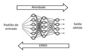
Figure 8: Schematics of the workings of the Backpropagation algorithm
