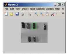
Figure 11 – Image of a parking place with the cut on a single spot (green rectangle).
