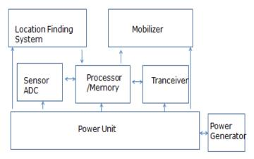
Figure 2. Components of a Sensor Node
