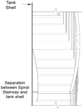
Fig. 19: Spiral Stairway Separated from the Tank Shell
