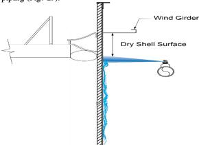
Fig. 24: Schematic of Dry Shell Surface
