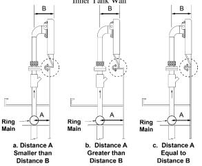
Fig. 48: Foam Pourer Installaton on Top Angle
