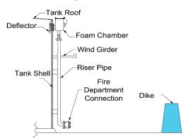
a. Semi-automatic System with Fire Department Connection Inside the Diked Area
