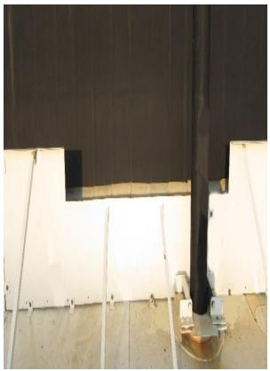
Fig. 8: Foam Dam Localized Height Modification
