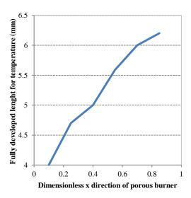
**Fig. 6:** Fully developed length of temperature versus porosity
