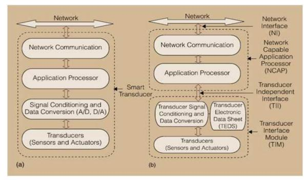
Figure 3: (a) Smart Transducer Model (b) This Architecture Adds TEDS and the System Partition into NCAP and TIM, with a TII
