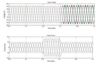
Figure 7: Supply Side Voltage and Supply Side Current with PQ Disturbances
