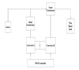
Figure 2: Block Diagram of UPQC
