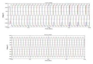
Figure 13: Simulated Results of UPQC (a) Load Voltage (b) Source Voltage
