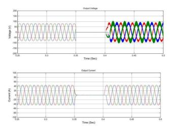
Figure 6: Load Side Voltage and Load Side Current with Interruption
