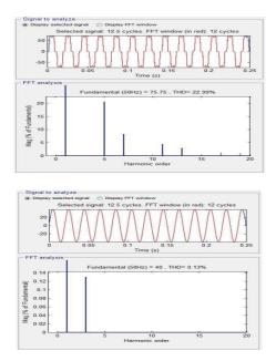
Figure 12: (a) THD Distorted Source Current (b) Compensated Source Current
