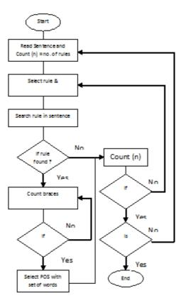
Figure 1: Flowchart for Extractor Process
