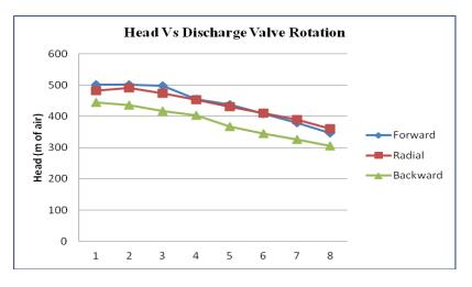
Fig. 5: Head Vs Discharge Valve Rotation of all blades.
