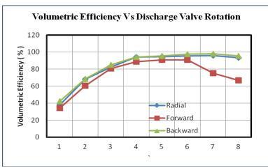
Fig. 3: Volumetric Efficiency Vs Discharge Valve Rotation of all blades.
