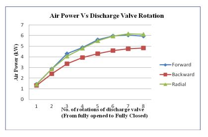
Fig. 4: Air Power Vs Discharge Valve Rotation of all blades.
