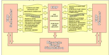
Figure 2. Closing the Planner/Scheduler Loop with simulation
