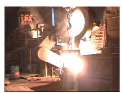
Figure 2 - Melting in induction furnace
