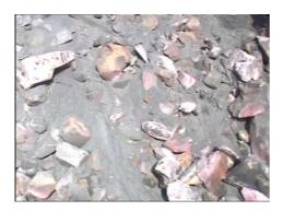
Figure 3b - Waste casting sand and slag
