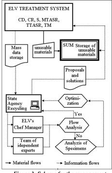
Figure 3- Scheme for the management of material flows
