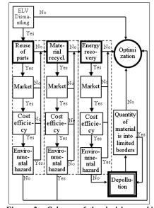
. Figure 2 - Scheme of the decision making model in the selection of operations with ELV
