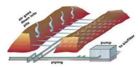
Figure 3. The aerated static pile
