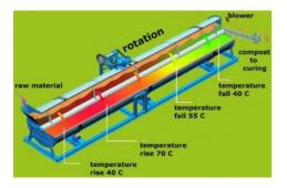
Figure 4. Rotary drum
