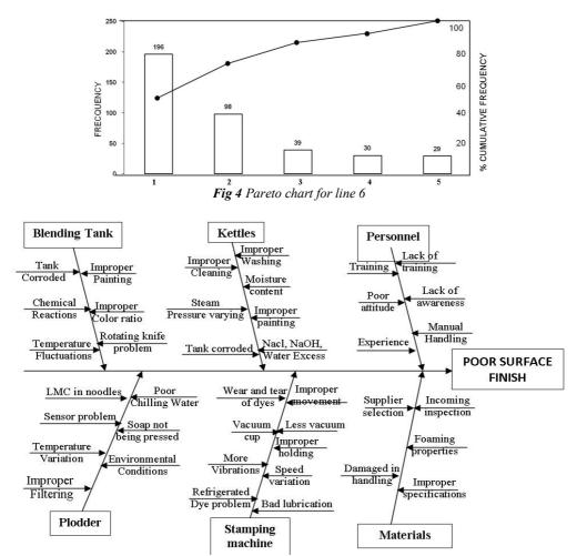
Fig 5 Cause and effect diagram for poor surface finish
