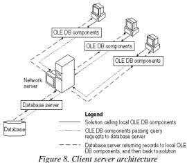
The client server model is based on the distribution of functions between the two types of independent and autonomous processes: server and client. The client is any process that requires specific services from server process. The server is a process that provides services to clients.
