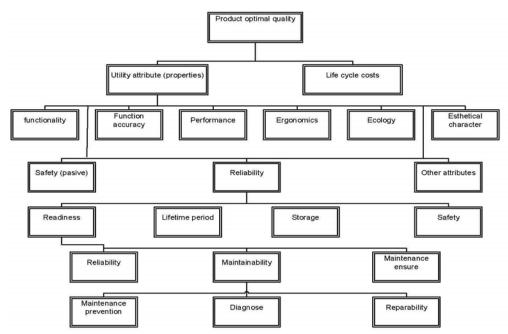
Figure 2 Criterions for evaluation of machine tool of quality and reliability
