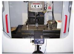
Figure. 3 Measurement using Laser interforometer
