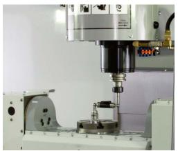
Figure 4 Measurement of geometrical inaccuracy of CNC machine tool
