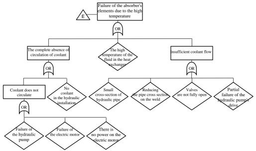
Figure 6. Sub failure tree for the peak event "Failure of the absorber's elements due to the high temperature"
