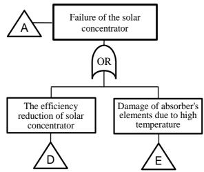
Figure 4. Fault tree of the solar concentrator
