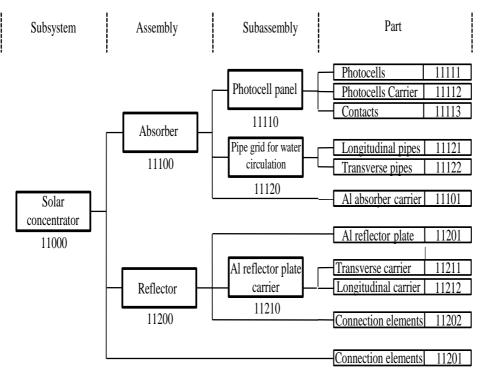
Figure 3. Scheme of dismembering of the solar concentrator
