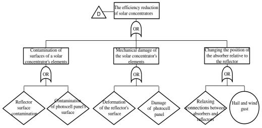
Figure 5. An independent sub fault tree for the peak event"Reduction of the solar concentrator's efficiency"
