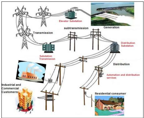
Figure 1 - Composite Power System Source: Schettino (2013 p.38)
