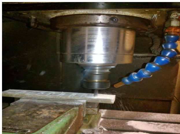
Figure 1: Machining of GFRP by CNC vertical machining center with K10 carbide End Mill
