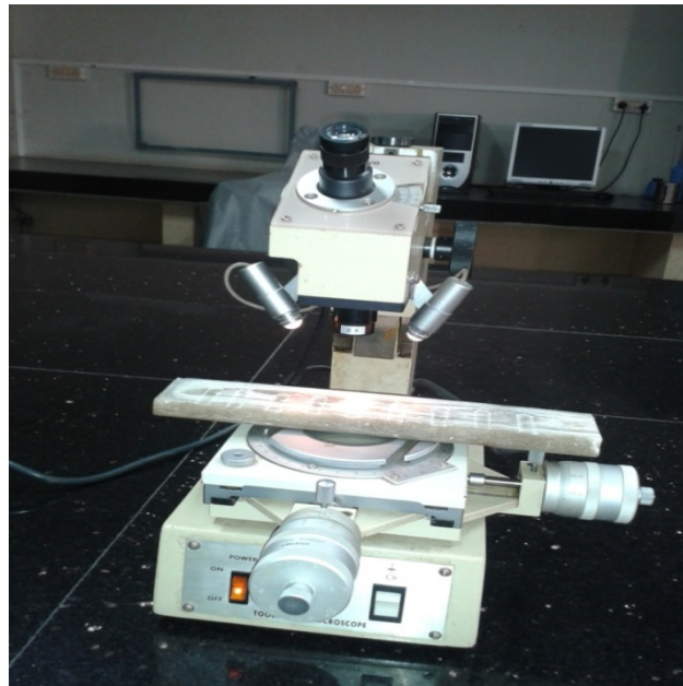
Figure 3: Measurement of delamination damage using Tool makers Microscope
