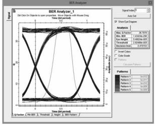
FIG. 12. MAX Q AND EYE PATTERN OF 1560 NM
