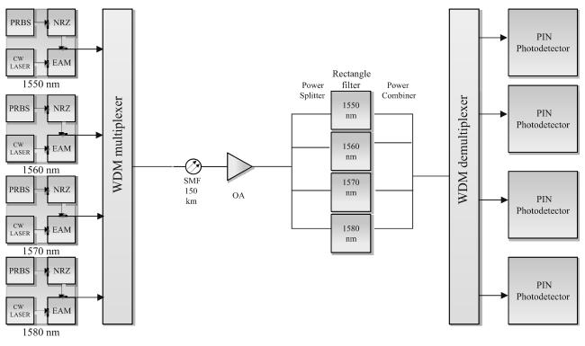
FIG. 7. PROPOSED MODEL OF WDM SYSTEM
