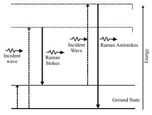
FIG. 2. RAMAN STOKES AND ANTI-STOKES SCATTERING
