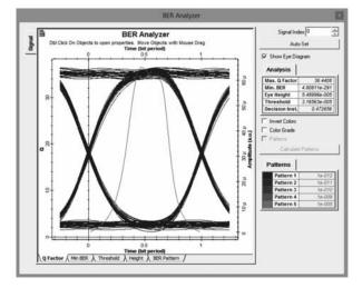
FIG. 11. MAX Q AND EYE PATTERN OF 1550 NM
