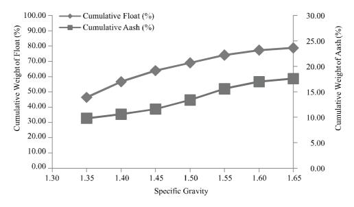
FIG. 4(a). WASHABILITY CURVES FOR SIZE FRACTION - 1.4+0.71mm SHOWING CHANGE IN ASH CONTENT
