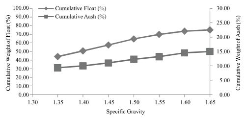
FIG. 3(a). WASHABILITY CURVES FOR SIZE FRACTION -0.71+0.5mm SHOWING CHANGE IN ASH CONTENT
