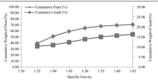
FIG. 6(a). WASHABILITY CURVES FOR SIZE FRACTION -5.6+3.35 mm SHOWING CHANGE IN ASH CONTENT
