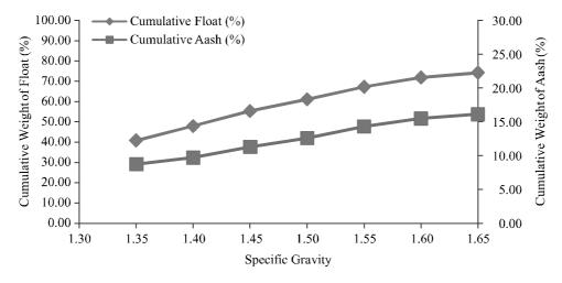
FIG. 2(a).WASHABILITY CURVES FOR SIZE FRACTION -0.5+0.3mm SHOWING CHANGE IN ASH CONTENT
