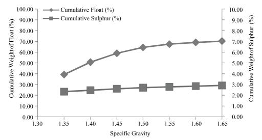
FIG. 6(b). WASHABILITY CURVES FOR SIZE FRACTION -5.6+3.35mm SHOWING CHANGE IN SULPHUR CONTENT
