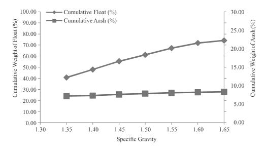
FIG. 2(b). WASHABILITY CURVES FOR SIZE FRACTION -0.5+0.3mm SHOWING CHANGE IN SULPHUR CONTENT
