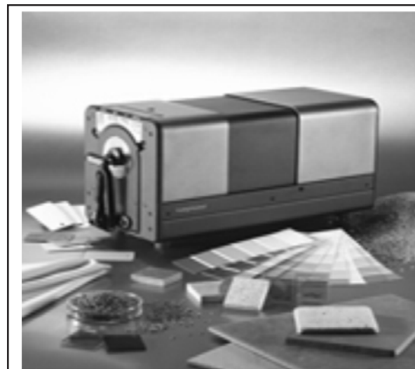
FIG. 1. SPECTROPHOTOMETER FOR MEASURING COLOURED TEXTILES
