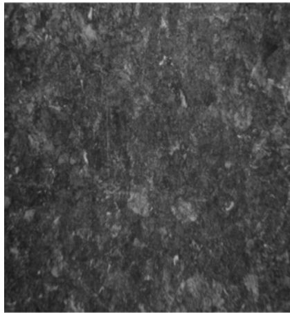
(a) PEARLITE IN AS RECEIVED SAMPLE
