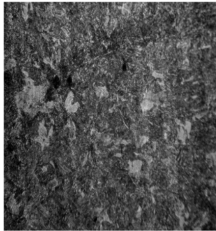
(b) UPPER BAINITE IN A SAMPLE AUSTEMPERED AT 400°C
