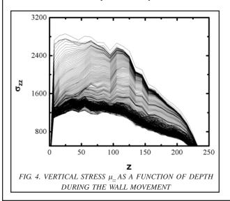
Janssen prediction. It is reported that the main reason for the splitting of stress profiles is the tangential force at the bead and the container wall. According to Janssen model the bead at the silo wall are at the coulomb yield criterion. Thus the presence of large number of beads far from the yield criterion gives rise to deviation of Janssen model.
