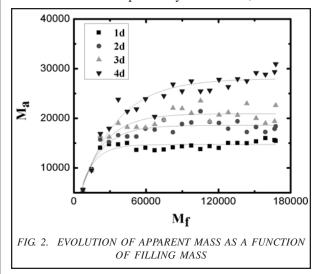
is the value of saturation mass. Thus with the increase in bead size the most of beads are away from coulomb criterion that gives rise to apparent mass and also variation in shielding of vertical stresses in granular columns.
