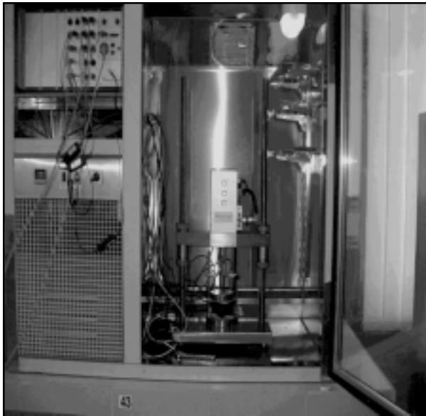
FIG. 2. UNIVERSAL TESTING MACHINE (UTM-5P)
