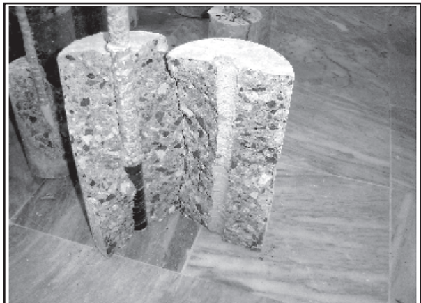
FIG. 8. CONCRETE KEY OF GFRP REBARS AFTER PULLOUT TESTS
