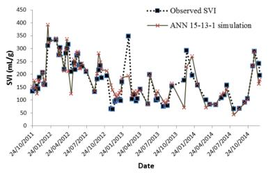
Figure 5: Observed and predicted sludge volume index in Batna wastewater treatment plant (2011-2014).
