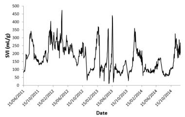
Figure 3: Change of SVI in Batna WWTP from June 15, 2011 to Dec. 31, 2014.
