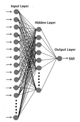
Figure 4: Proposed Multi-Layer Feed Forward Network architecture.
