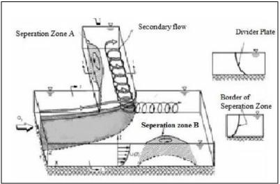
Figure 1: Flow algorithm through intake structure
