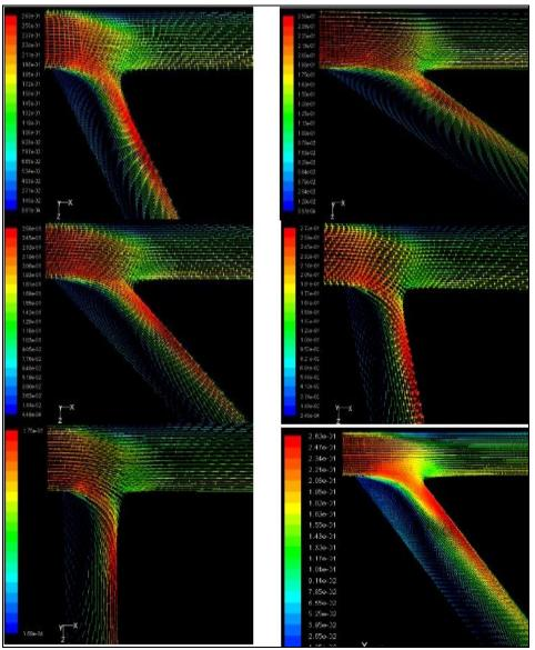
**Figure 5:** Flow stream at inlet point at 0.02m above bottom with diverting angle: 30, 15, 90° and at left side from down to up diverting angle 60°, 45°, 35°
