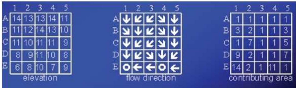
Fig 1. Diagram Showing D8 Algorithm method, e.g. for pixel A1, there are three surrounding cells (A2, B1 and B2) and the least of among them is B1, so the flowpath southward and downward. for pixel C3, the least of all 8 nearby pixel is D2, so the is southwest towards lower-left. Cells E1 and E4 don't have lower neighbors there are thus "sink".
